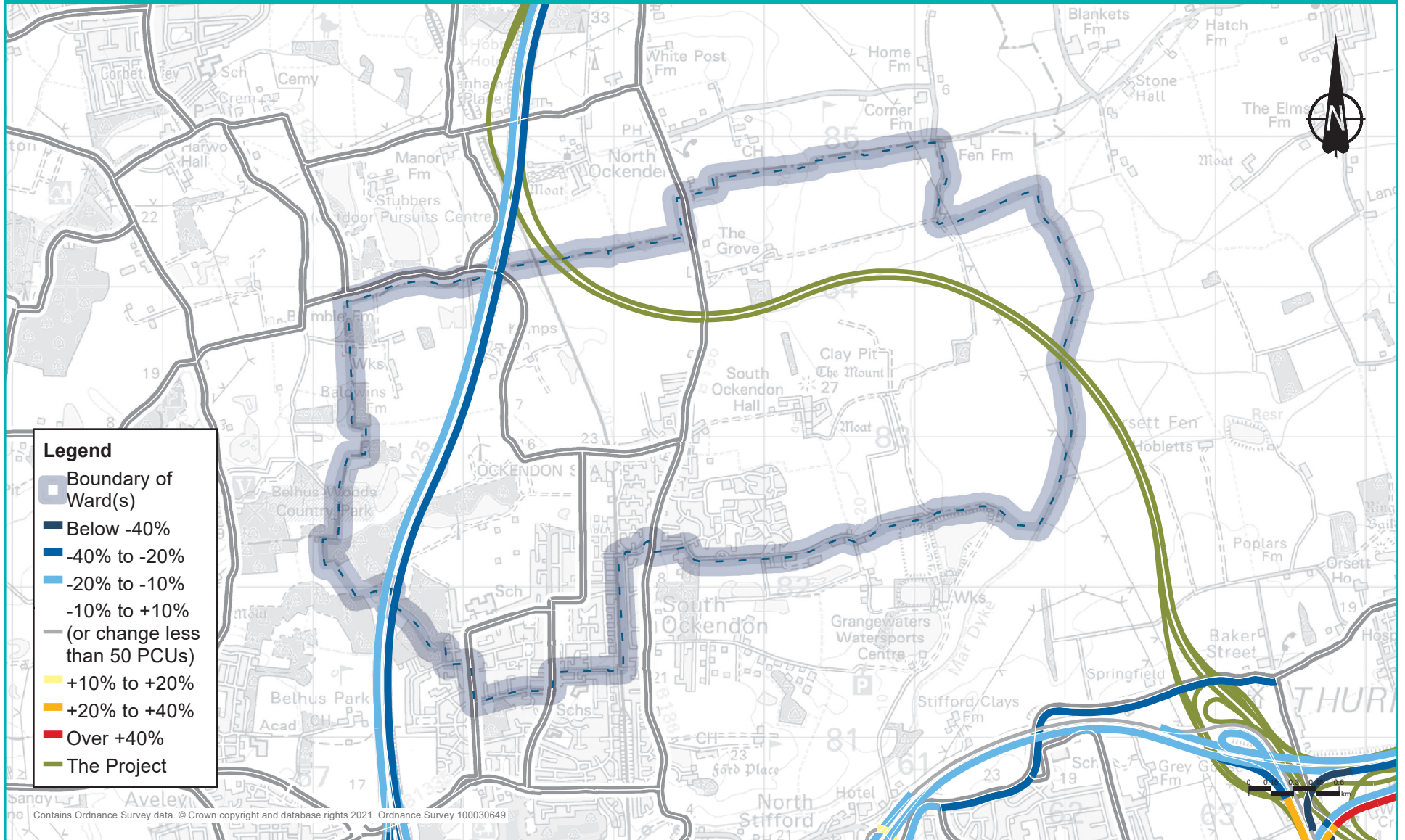
Figure 20.10: Predicted percentage change in traffic flows with the new road during the evening peak in 2029
