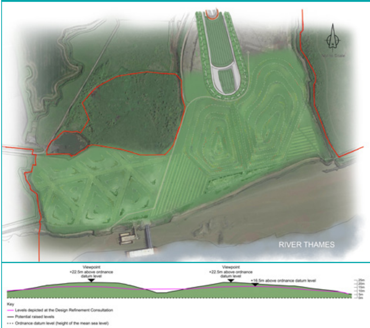
Figure 3-2 Proposed changes in the form and height of the earthworks at Tilbury Fields
