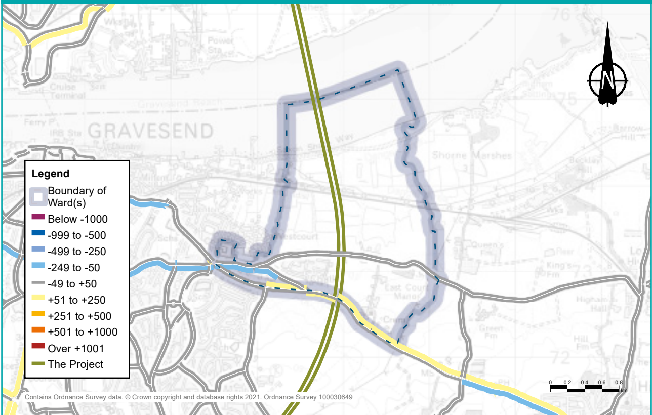
Figure 4.4: Predicted change in traffic flows (PCUs) with the project during the morning peak, 2029
