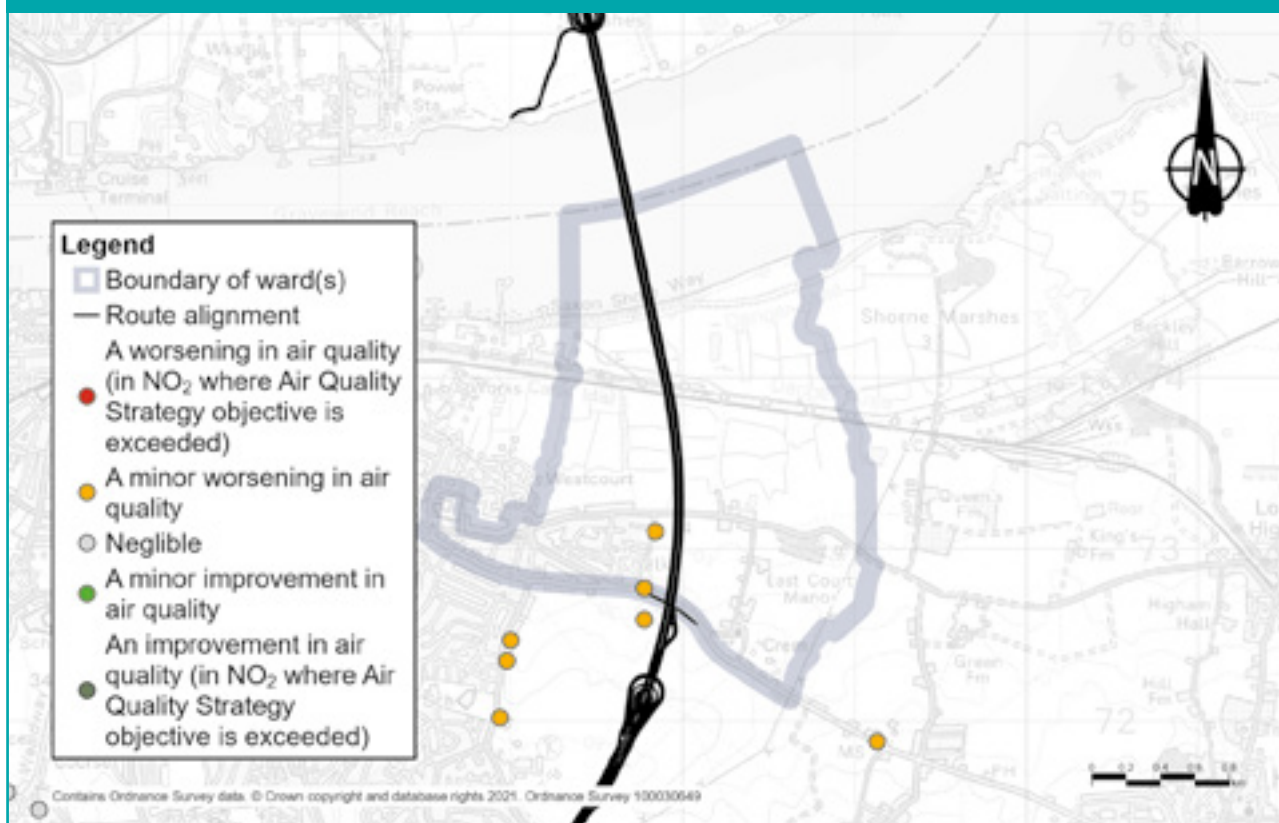
Figure 4.19: Predicted changes in NO 2 levels within Chalk ward once the new road is open
