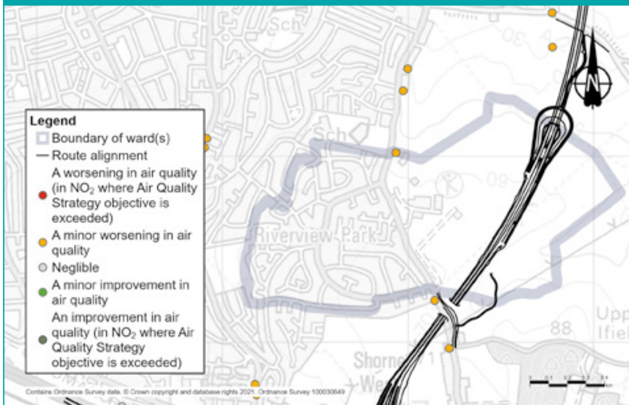
Figure 7.18: Predicted changes in NO 2 levels within Riverview ward once the new road is open
