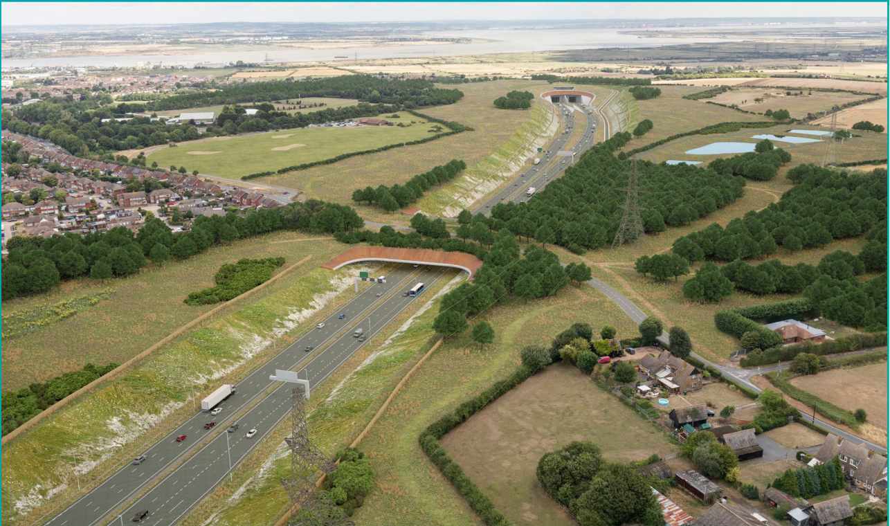
Figure 5-7. Community impacts consultation – proposed Thong Lane green bridge linking Gravesend and Thong and the approach to the southern tunnel entrance, looking north
